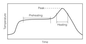
For soldering (Example : Sn/Pb)
