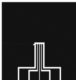
(Fig .1) Glass-Epoxy Board coated Copper FR-4 25.4 × 25.4 × 0.8 ( Unit ; mm )
