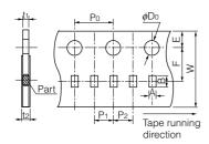
Embossed Carrier Tape Dimensions in mm (not to scale)
