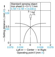
The graph on the left is plotted with the sensitivity adjusted so as to just detect a  $5 \times 5 \times t$  1 mm  $0.197 \times 0.197 \times t$  0.039 in iron sheet placed at a distance of 0.6 mm 0.024 in.
