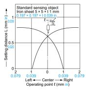
The graph on the left is plotted with the sensitivity adjusted so as to just detect a  $5 \times 5 \times t$  1 mm  $0.197 \times 0.197 \times t$  0.039 in iron sheet placed at a distance of 0.8 mm 0.031 in.
