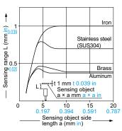
As the sensing object size becomes smaller than the standard size (iron sheet  $5 \times 5 \times t$  1 mm  $0.197 \times 0.197 \times t$  0.039 in), the sensing range shortens as shown in the left figure.
