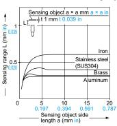
As the sensing object size becomes smaller than the standard size (iron sheet 5 × 5 × t 1 mm  $0.197 \times 0.197 \times t 0.039$  in), the sensing range shortens as shown in the left figure.
