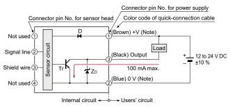
Note: The quick-connection sub cable does not have +V (brown) and 0 V (blue). The power is supplied from the connector of the main cable.
