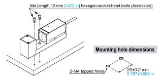
Mount the controller using 2 pcs. M4 pan head screws, with a tightening torque of 1.2 N·m or less.
