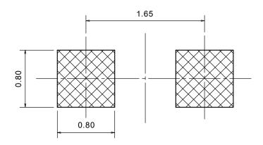
(Note1)Electrode projection is not included in the package dimensions. (Note2)About solder thickness, please examine the products yourself completely. (Recommended thickness:  $t=0.10 \text{ mm} \sim 0.15 \text{ mm}$ )
