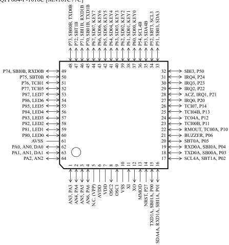
Note) Pin 5 serves as the VPP pin in the MN101CF77G, and cannot be used as a user pin.
