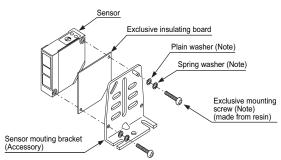
Note: Attached with the exclusive insulating board.
