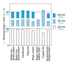
These bars indicate the sensing range with the respective objects when the distance adjuster is set to a sensing range of 40 mm 1.575 in, 30 mm 1.181 in and 20 mm 0.787 in long, respectively, with white non-glossy paper.
