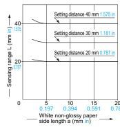
These curves show the characteristics with the maximum sensing range set to 40 mm 1.575 in, 30 mm 1.181 in and 20 mm 0.787 in, with white non-glossy paper (10 × 10 mm  $0.394 \times 0.394$  in).
