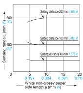
These curves show the characteristics with the maximum sensing range set to 200 mm 7.874 in. 100 mm 3.937 in and 40 mm 1.575 in, with white non-glossy paper (20 × 20 mm  $0.787 \times 0.787$  in).
