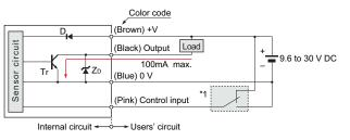
Symbols ... D : Reverse supply polarity protection diode ZD: Surge absorption zener diode Tr : NPN output transistor
