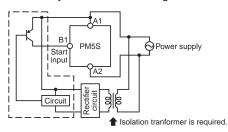
• Input and Power supply circuit
