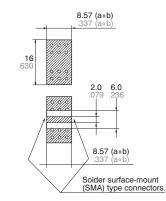
Material: Glass PTFE double-sided through hole PC board R-4737 (Matsushita Electric Works) Board thickness: t = 0.8 mm .031 inchCopper plating:  $18 \mu \text{m}$ Connector (SMA type receptacle) Product name: 01K1808-00 (Waka Manufacturing Co., Ltd.) Value has compensation PC board subtracted only for insertion loss. (Eliminate loss of connector and PC board.)
