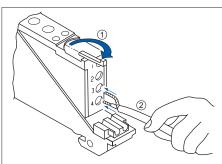
①Rotate the cable lock lever approx. 160° clockwise.
