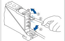
③ Rotate the cable lock lever approx. 90° counterclockwise. (The beam-receiving cable is hooked up.)
