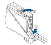
® Rotate the cable lock lever back to the "LOCK" position. (The beam-emitting cable is hooked up.)
