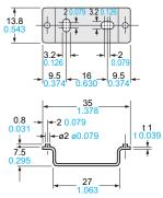
Material: Cold rolled carbon steel (SPCC) (Uni-chrome plated)
