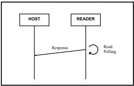
AUTOSEND/AUTONOTIFY mode are enabled, a response is automatically transmitted at time of card inserted and card read.
