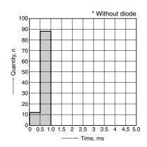
7.-(1) Electrical life test (at resistive load) Sample: CP1-12V Quantity: n = 4 (N.C. = 2, N.O. = 2) Load: Resistive load (N.C. side: 10A 14V DC, N.O. side: 20A 14V DC) Operating frequency: ON 1s, OFF 9s Ambient temperature: Room temperature
