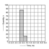
6. Distribution of release time Sample: CP1-12V, 100pcs Ambient temperature: 20°C 68°F
