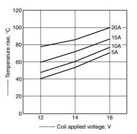
1.-(2) Coil temperature rise (85°C 185°F) Sample: CP1-12V, 6pcs Point measured: Inside the coil Contact carrying current, 5A, 10A, 15A, 20A Resistance method, ambient temperature 85°C 185°F
