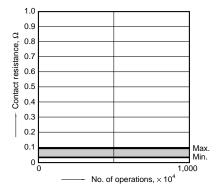
2-(2). Change in dynamic contact resistance (10 μA 1 mV DC resistive load) Tested sample: ASX20012, 10 pcs.
