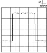
6-(3). Electrical life test (Motor lock)
