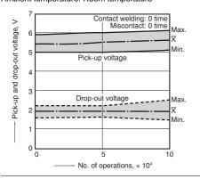
7-(2). Electrical life test (Motor free) Sample: JJM1-12V, 6pcs. Load: Inrush 25A, Steady 5A, Brake current 18A 14V
