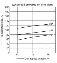
1.-(6) Coil temperature rise (at 85°C 185°F) Sample: ACJ5212, 3pcs Measured portion: Inside the coil Contact carrying current: 10A, 15A, 20A Ambient temperature: 85°C 185°F
