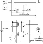
Load current waveform Inrush current: 25A, Steady current: 6A, Brake current: 13A
