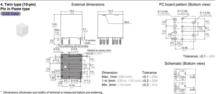
Intervals between terminals is measured at A surface level.
