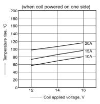
1.-(2) Coil temperature rise (at 85°C 185°F) Sample: ACJ1212, 3pcs Measured portion: Inside the coil Contact carrying current: 10A, 15A, 20A Ambient temperature: 85°C 185°F
