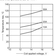
1-(2). Coil temperature rise Sample: ACNM7112, 3pcs Measured portion: Inside the coil Contact carrying current: 10A, 20A Ambient temperature: 110°C 230°F
