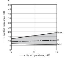
4-(2). Electrical life test (TV-8 type) (8A 277V AC, resistive load) Sample: LKQ1aF-12V-TV8, 6 pcs. Operation frequency: 20 times/min. (ON/OFF = 1.5s: 1.5s)Ambient temperature: 20°C 68°F
