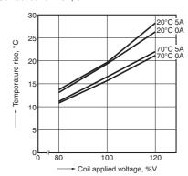
2-(2). Coil temperature rise (TV-8 type) Sample: LKQ1aF-12V-TV8, 6 pcs. Point measured: coil inside Contact current: 0A, 8A
