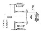
Recommended metal mask pattern Metal mask thickness: When 120 μm (Terminal portion opening area ratio: 66%) (Metal portion opening area ratio: 100%)
