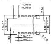
Recommended metal mask pattern Metal mask thickness: When 120 μm (Terminal portion opening area ratio: 66%) (Metal portion opening area ratio: 100%)
