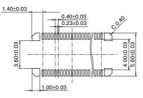
Recommended metal mask pattern Metal mask thickness: When 150  $\mu$ m (Terminal portion opening area ratio: 53%) (Metal portion opening area ratio: 100%)
