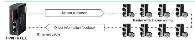
High speed network and high performance servo bring synchronous control
