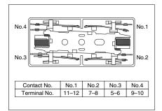
The table below shows the state of the other contacts when the current through the welded form "a" contact is 0 V and the rated voltage is applied through the form "b" contact.
