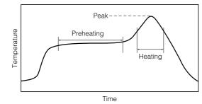
Recommended soldering conditions for flow
