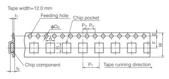
Taping condition: Lack of products in the middle of taping should be one MAX, but total quantity specified in the specifications should be secured.
