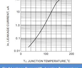
Fig.2 Leakage Current VS. Junction Temperature
