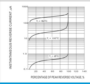
Fig.3 TYPICAL REVERSE CHARACTERISTIC
