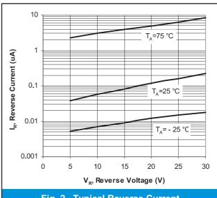
Fig. 2. Typical Reverse Current
