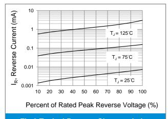
**Fig.3 Typical Reverse Characteristics**
