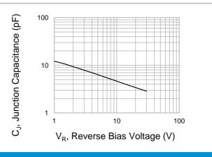
**Fig.2 Typical Junction Capacitance**
