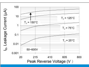
Fig.3 Typical Reverse Characteristics
