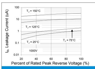
**Fig.4 Typical Reverse Characteristics**
