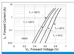
**Fig.6 Typical Forward Characteristics**
