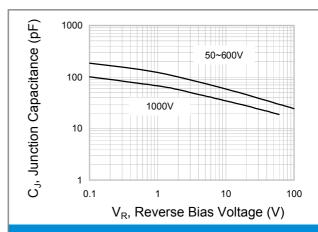
**Fig.2 Typical Junction Capacitance**
