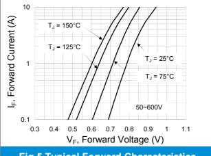
**Fig.5 Typical Forward Characteristics**
