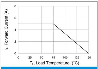
**Fig.1 Forward Current Derating Curve**
