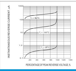
Fig.3 TYPICAL REVERSE CHARACTERISTIC
