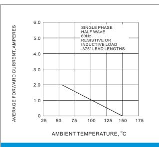
Fig.2 FORWARD CURRENT DERATING CURVE
