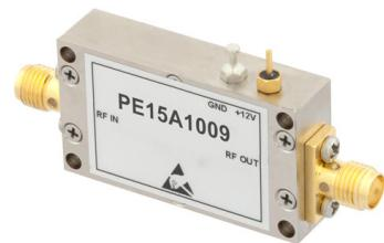
25 dBm IP3, 1.4 dB NF, 11 dBm P1dB, 10 MHz to 3 GHz, Low Noise Amplifier, 34 dB Gain, SMA
