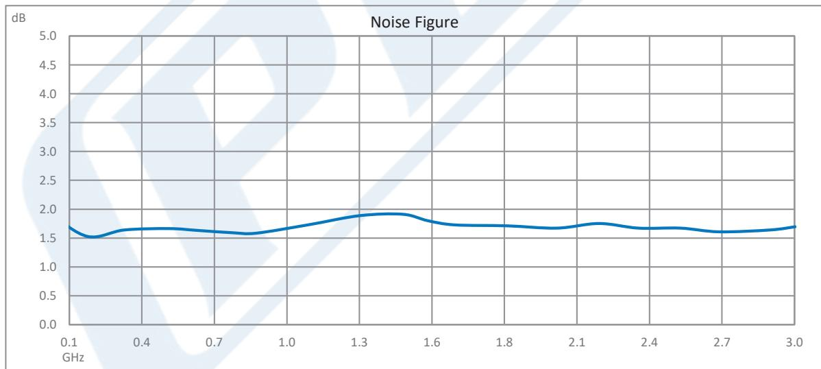
Click the following link (or enter part number in "SEARCH" on website) to obtain additional part information including price, inventory and certifications: [Input Protected Low Noise Amplifier, 20 MHz to 3000 MHz, 1 Watt RF Input Power, 25 dB Gain, 1.7 dB Noise Figure, 12V, SMA PE15A63016](#)
