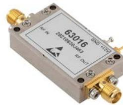
**Input Protected Low Noise Amplifier, 20 MHz to 3000 MHz, 1 Watt
