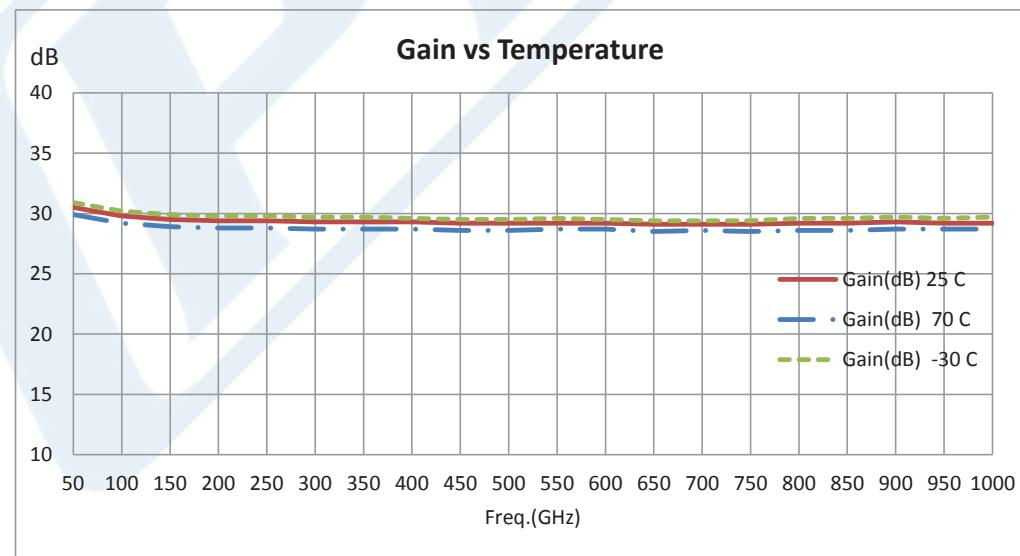
Click the following link (or enter part number in "SEARCH" on website) to obtain additional part information including price, inventory and certifications: [28 dBm P1dB, 50 MHz to 1 GHz, Medium Power GaAs Amplifier, SMA Input, SMA Output, 26 dB Gain, 5 dB NF PE15A4009](#)
