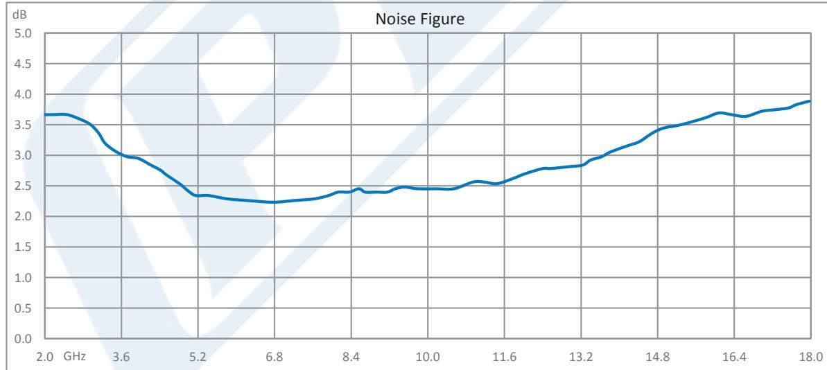
Click the following link (or enter part number in "SEARCH" on website) to obtain additional part information including price, inventory and certifications: [3 dB NF, 15 dBm P1dB, 2 GHz to 18 GHz, Low Noise Broadband Amplifier, 33 dB Gain, SMA PE15A3258](#)
