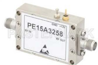
3 dB NF, 15 dBm P1dB, 2 GHz to 18 GHz, Low Noise Broadband Amplifier, 33 dB Gain, SMA
