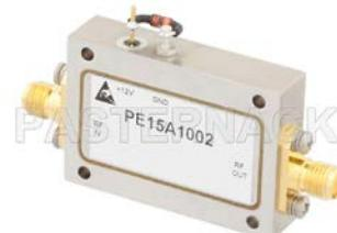
2 dB NF, 20 mW, 4 GHz to 8 GHz, Low
