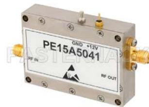
6 Watt P1dB, 800 MHz to 960 MHz, High Power Amplifier,
