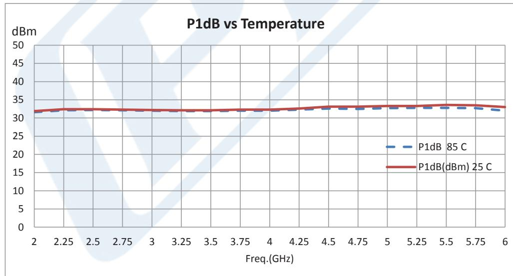
Click the following link (or enter part number in "SEARCH" on website) to obtain additional part information including price, inventory and certifications: [1 Watt P1dB, 2 GHz to 6 GHz, Medium Power Broadband Amplifier, 33 dB Gain, 39 dBm IP3, 5 dB NF, SMA PE15A4005](#)
