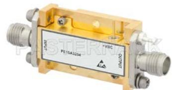
3 dB NF, 20 dBm P1dB, 30 MHz to 20 GHz, Low Noise Broadband Amplifier, 15 dB Gain, SMA
