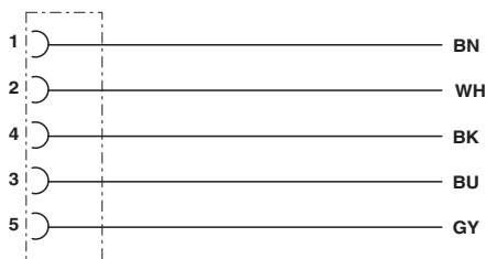
Contact assignment of the M12 socket
