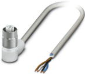
Sensor/Actuator cable, 4-position, PP-EPDM halogen-free, Gray RAL 7035, Free cable end, on Socket angled M12, A-coded, Cable length: 5 m, Hygienic design, With high-grade steel knurl
