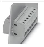
Panel feed-through terminal block, Connection method: Screw connection, Load current : 76 A, Cross section: 0.5 mm<sup>2</sup> - 16 mm<sup>2</sup>, AWG 20 - 6, Connection direction of the conductor to plug-in direction: 0 °, Width: 10.1 mm, Color: gray
