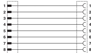
Contact assignment of M12 connector/socket
