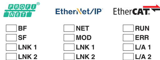
Figure 30 LED status indicators for PROFINET, EtherNet/IP™, EtherCAT®
