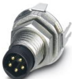
Sensor/actuator flush-type plug-in connector, plug, 5-pos., DeviceNet, M8, rear/screw mounting with M10 fastening thread, with straight solder connection
