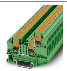
Feed-through terminal block, nom. voltage: 1000 V, nominal current: 41 A, connection method: Push-in connection, Rated cross section: 6 mm², cross section: 0.5 mm² - 10 mm², mounting type: NS 35/7,5, NS 35/15, color: green
