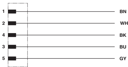
Contact assignment of the M12 plug
