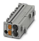
Marshalling patchboard, Nom. voltage: 500 V, Nominal current: 17.5 A, Cross section: 0.14 mm² - 2.5 mm², AWG: 12 - 26, Connection type: Push-in connection, Number of positions: 1, Number of connections: 4, Width: 11 mm, Length: 8.6 mm, Color: gray, Color of connection elements: black, Assembly: for snapping onto a DIN rail adapter, for snapping onto a cover flange
