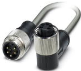
Bus system cable, DeviceNet, 5-position, PUR, Gray RAL 7001, Plug straight 7/8"-16UNF, on Socket angled 7/8"-16UNF, Cable length: 15 m
