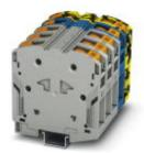
High-current terminal block, Blocked, Connection method: Power-Turn connection, Cross section: 10 mm² - 70 mm², AWG: 8 - 2/0, Width: 80 mm, Color: gray/blue, Mounting type: NS 35/15
